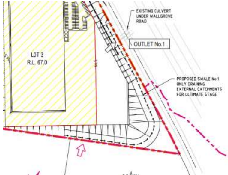
Figure 5 Swale Extract from Gazcorp Industrial Estate Stormwater Concept Plan (Approved Design)
