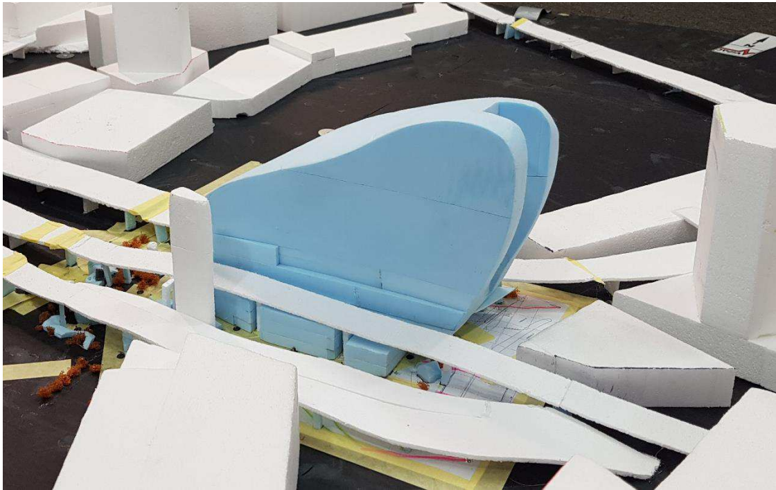
Figure 5: Close up view of the 1:400 model of the proposed development in the wind tunnel (proposed design).
