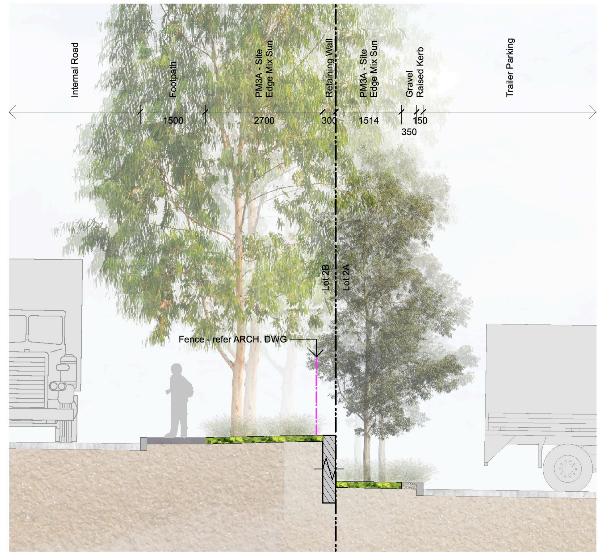
03 Southern Boundary Typical Section - Scale 1:50 @ A1
