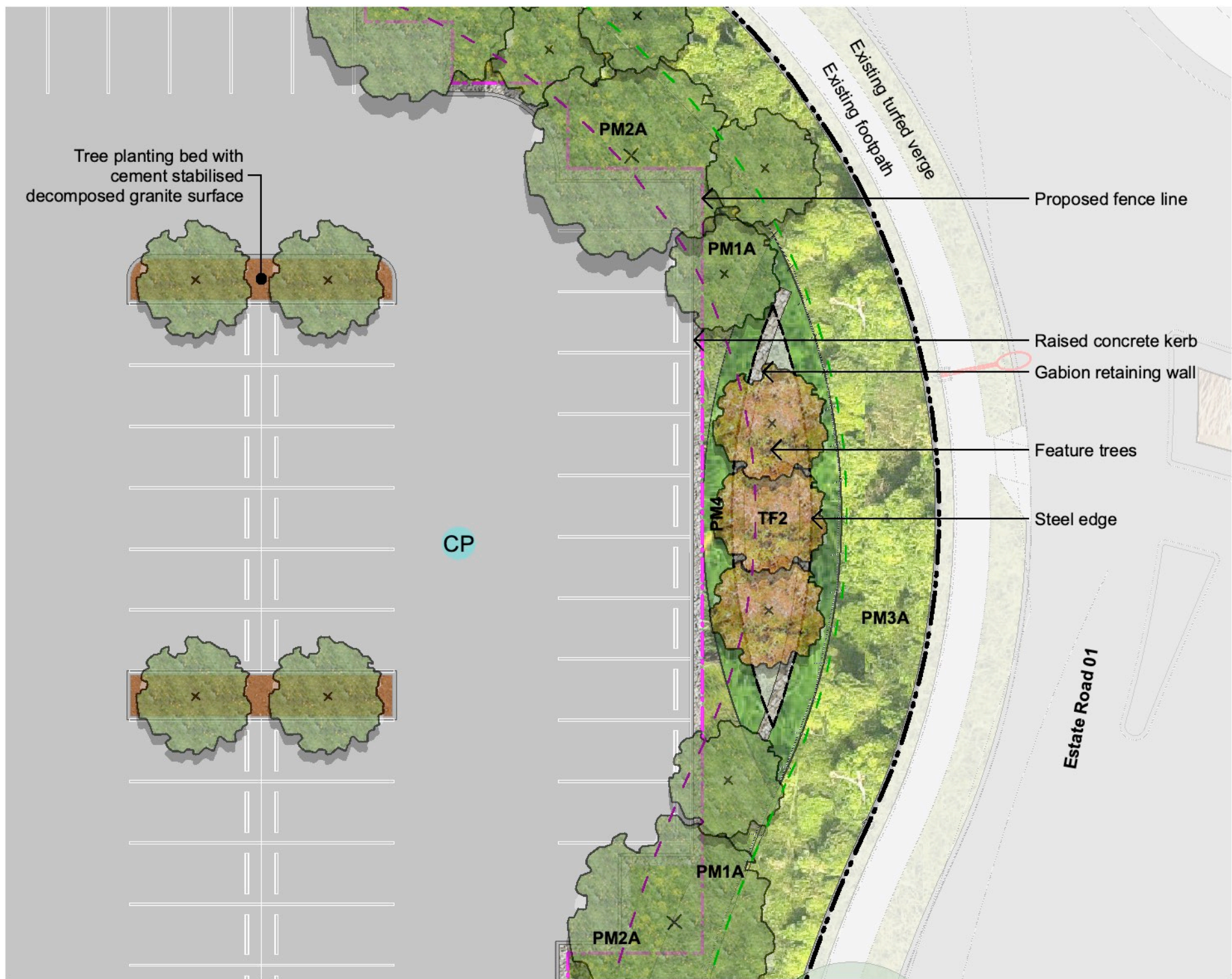
01 Carpark - Site Marker Detail Plan - Scale 1:200 @ A1
