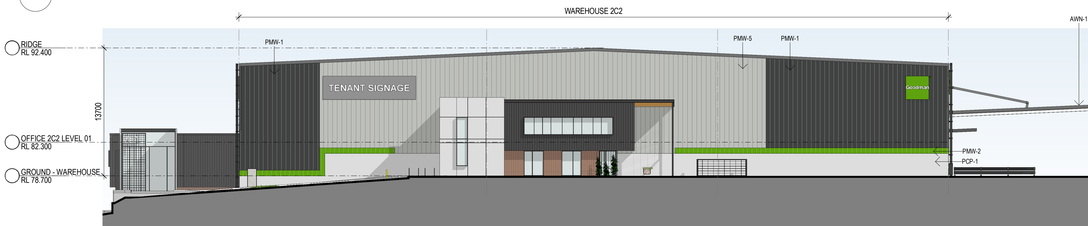
4 ELEVATION SOUTH - WAREHOUSE 2C 1 : 250
