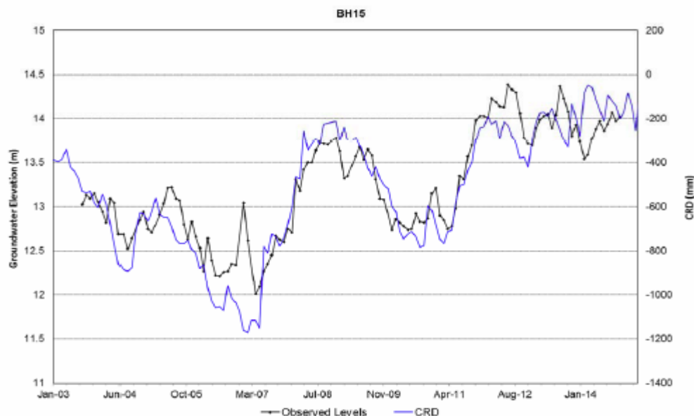
Figure 3. Strong evidence of rainfall recharge at a shallow coal monitoring site (BH15)
