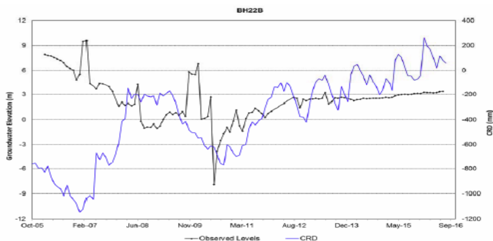
Figure 8. Hydrographic correlation at BH22B (over LW4/5) initially with mining and then with rainfall
