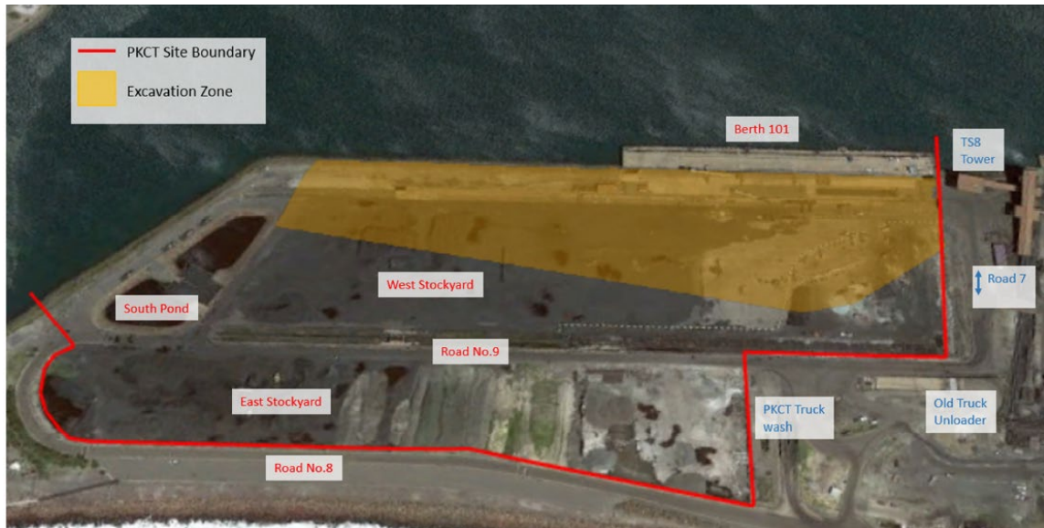
Figure 2.3 Proposed excavation zone within MBD Site Compound
