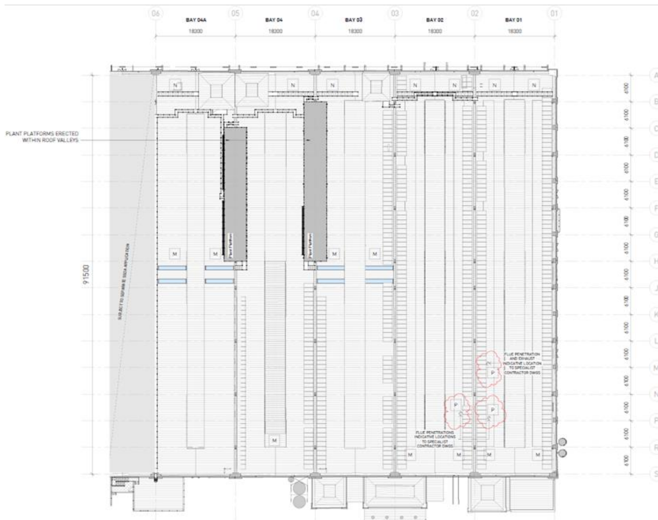
Figure 2 Proposed Roof Plan identifying the location of the flues
