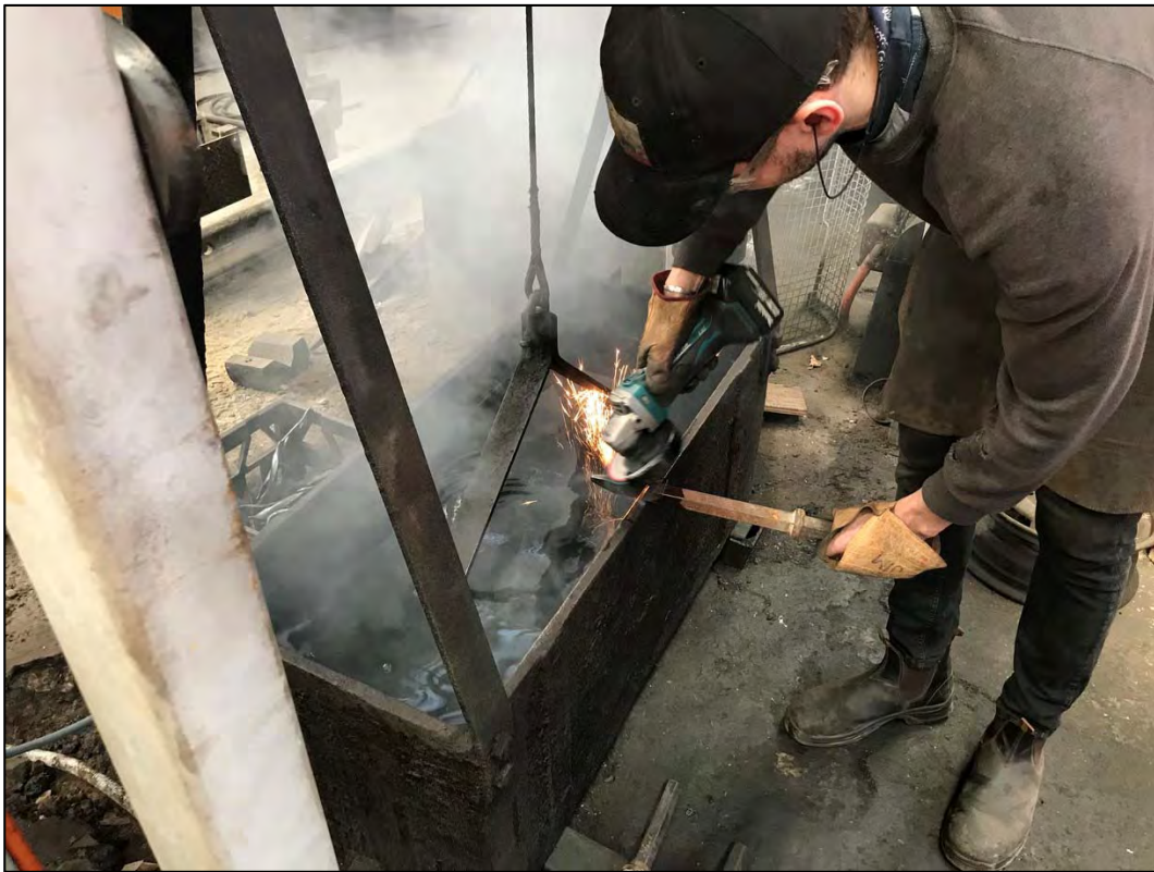
Photograph 9: Ineffective exhaust ventilation of smoke generated during oil quenching, particularly when smoke is laterally dispersed as cooling steel is grinded.
