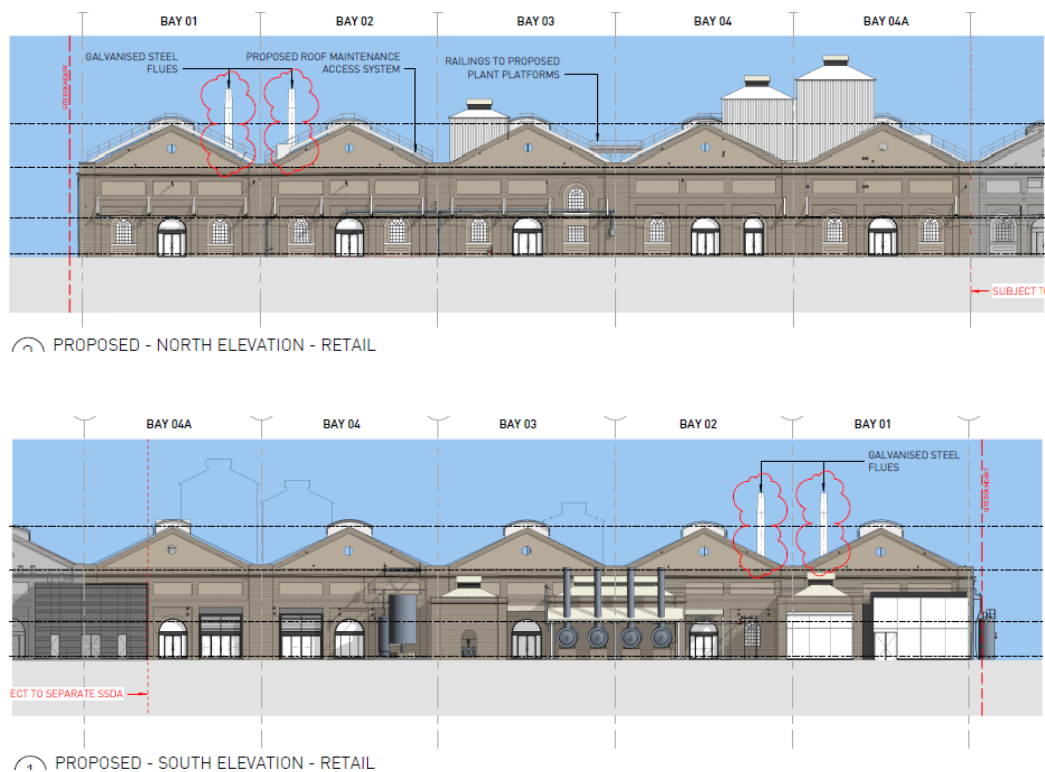
Figure 4 Proposed elevations of Bays 1-4a
