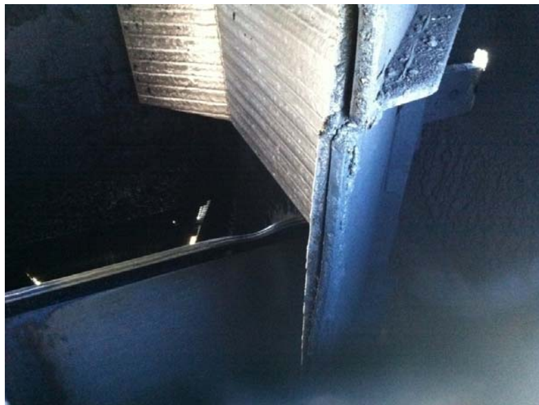
Figure 6.2: View of impact plate, diverter gates and side wear-plates
