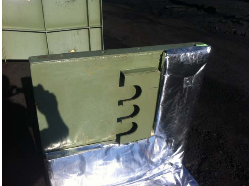
Figure 6.7: View of internal mounting plate for impact plate shaft support
