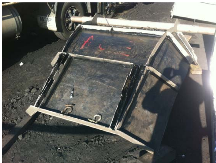
Figure 6.1: Impact plate with rear surface coated with rubber
