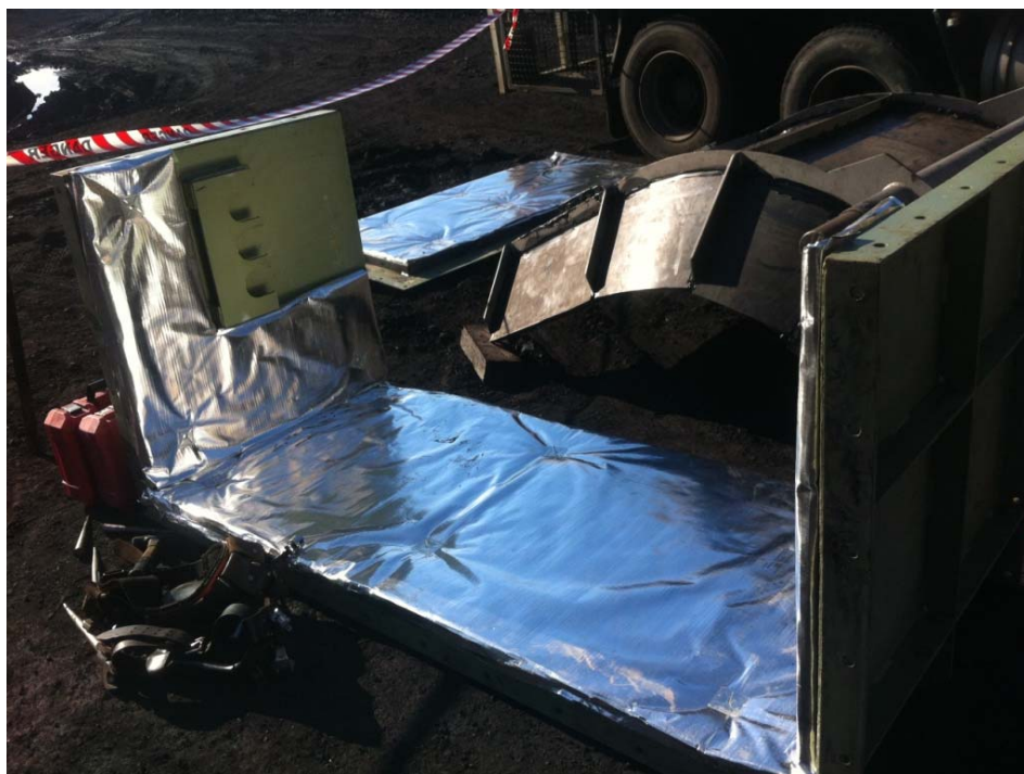
Figure 6.13: Aluminium foil-faced Absorptive lining inside enclosure cover
