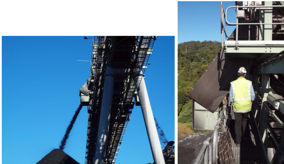
Figure 6.10: Photographs of parts of the trouser leg discharge chutes
