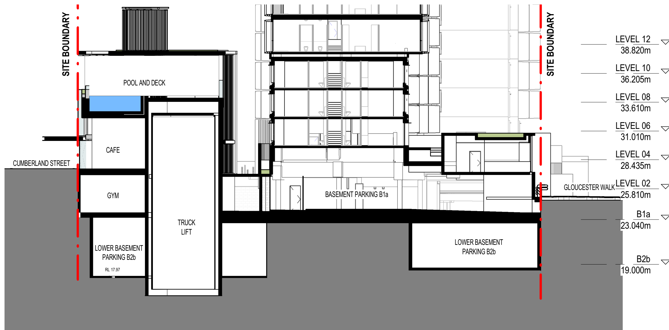
2 GA CROSS SECTION CUMBERLAND AND UNITS
