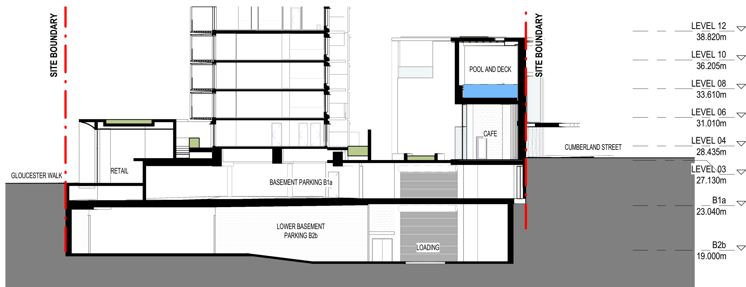
3 GA CROSS SECTION BASEMENTS
