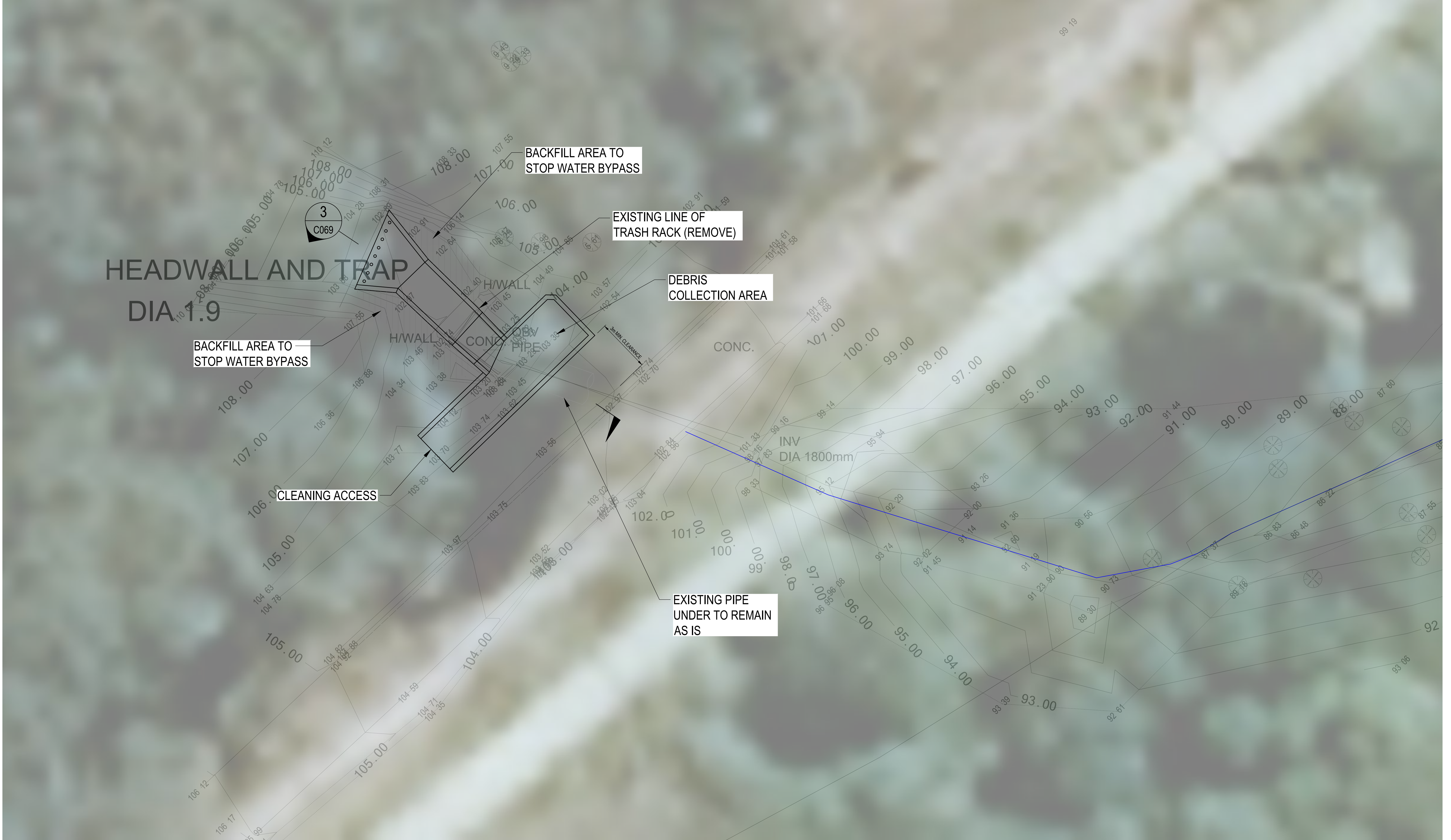
UPPER CONVEYOR CULVERT AND TRASH RACK SCALE: 1:100
