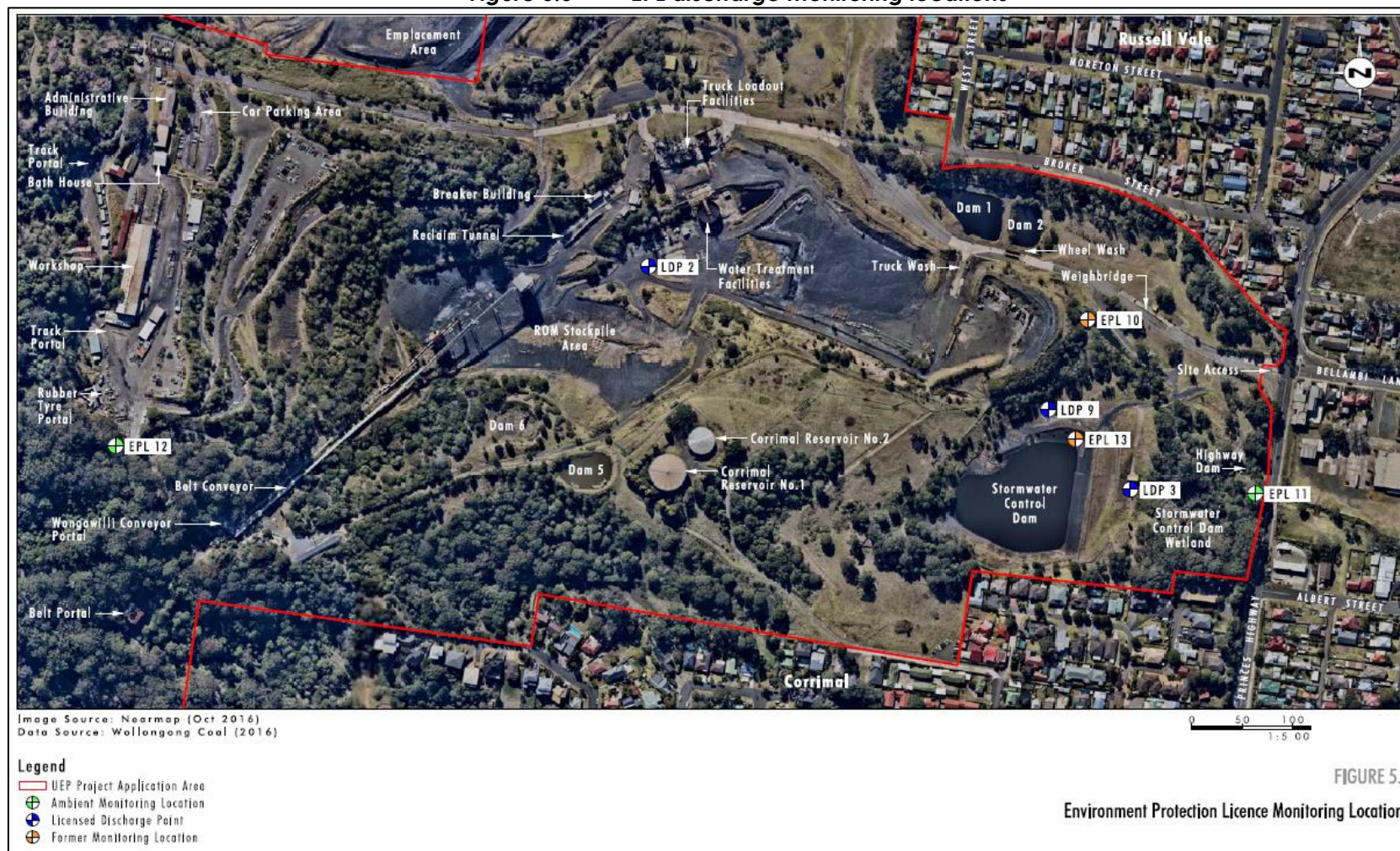
Figure 5.5 EPL discharge monitoring locations
