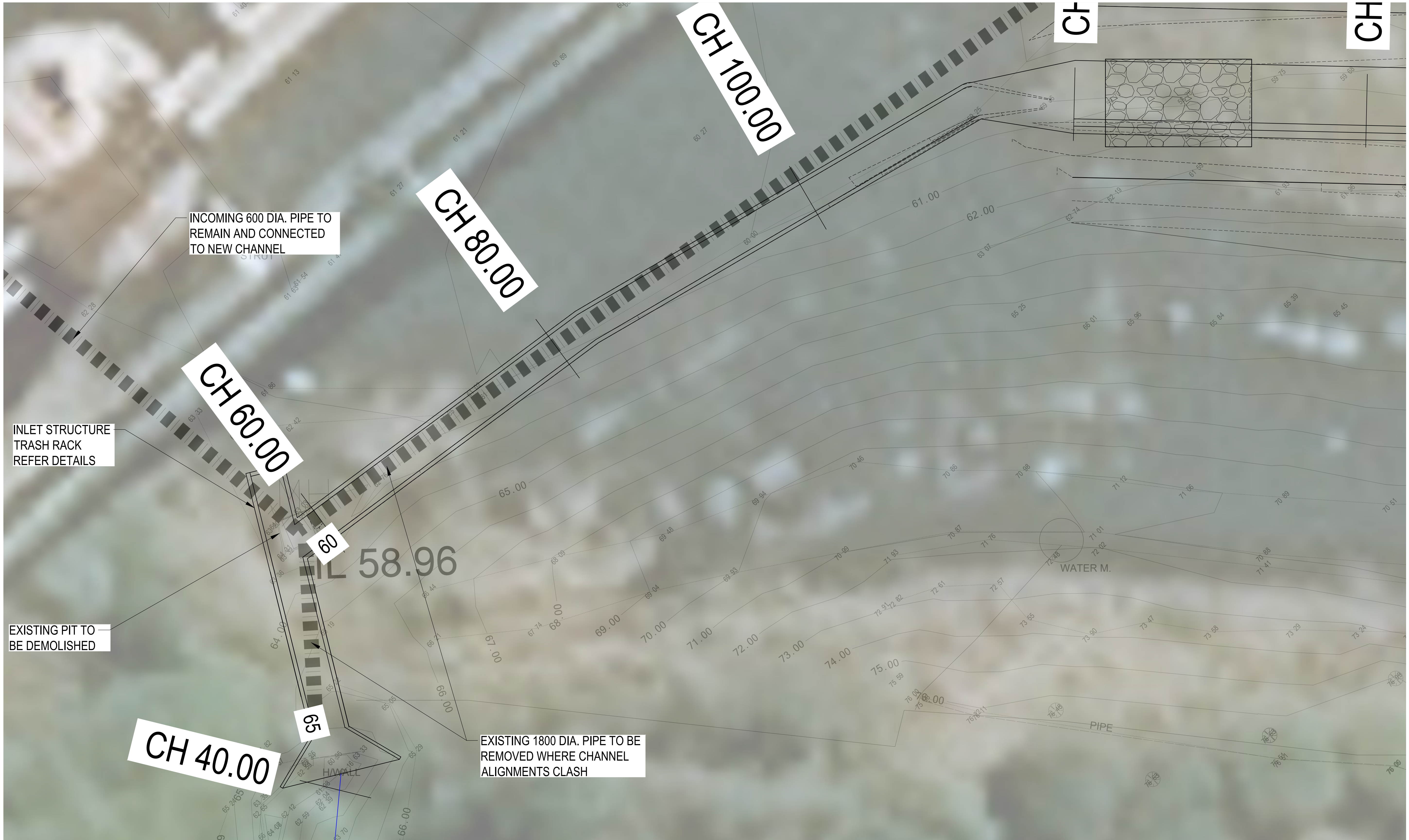
DIVERSION CHANNEL DETAIL PLAN CH 40.00 to CH 140.00 SCALE: 1:200
