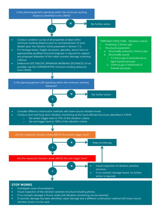
Figure 8: Monitoring protocol for structural damage
