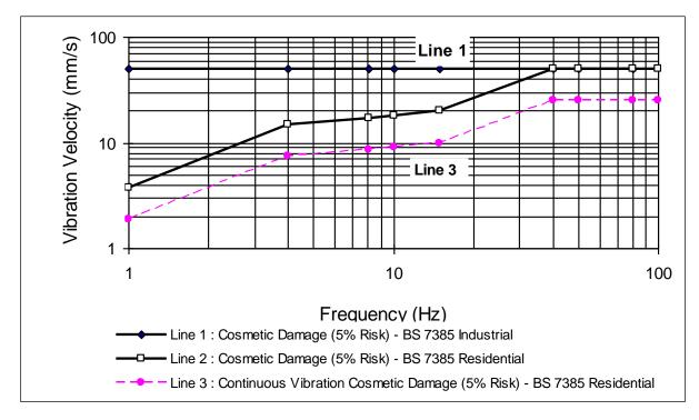
Figure 2: Graph of Transient Peak Component Particle Velocity Vibration Guide Values for Cosmetic Damage
