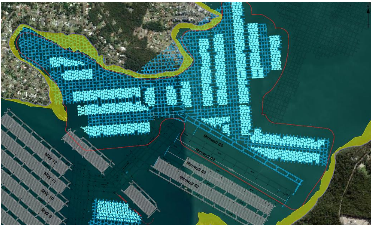
Figure 2 - Predicted Subsidence impact areas due to extraction of S2 - S5 panels and pillar secondary extraction (Hill, 2020)
