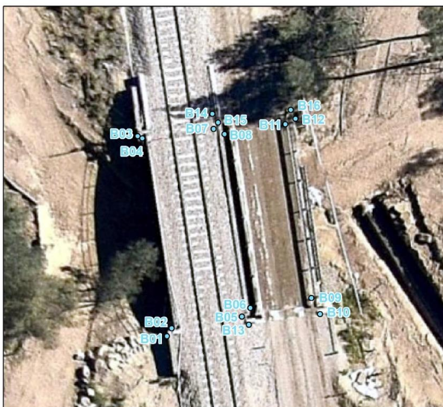
Figure 8-3 Locations of the 3D monitoring points for the Bridges
