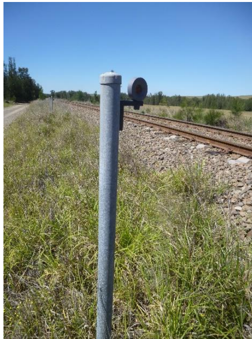
Figure 8-2 Prism arrangement for the PH-Line
