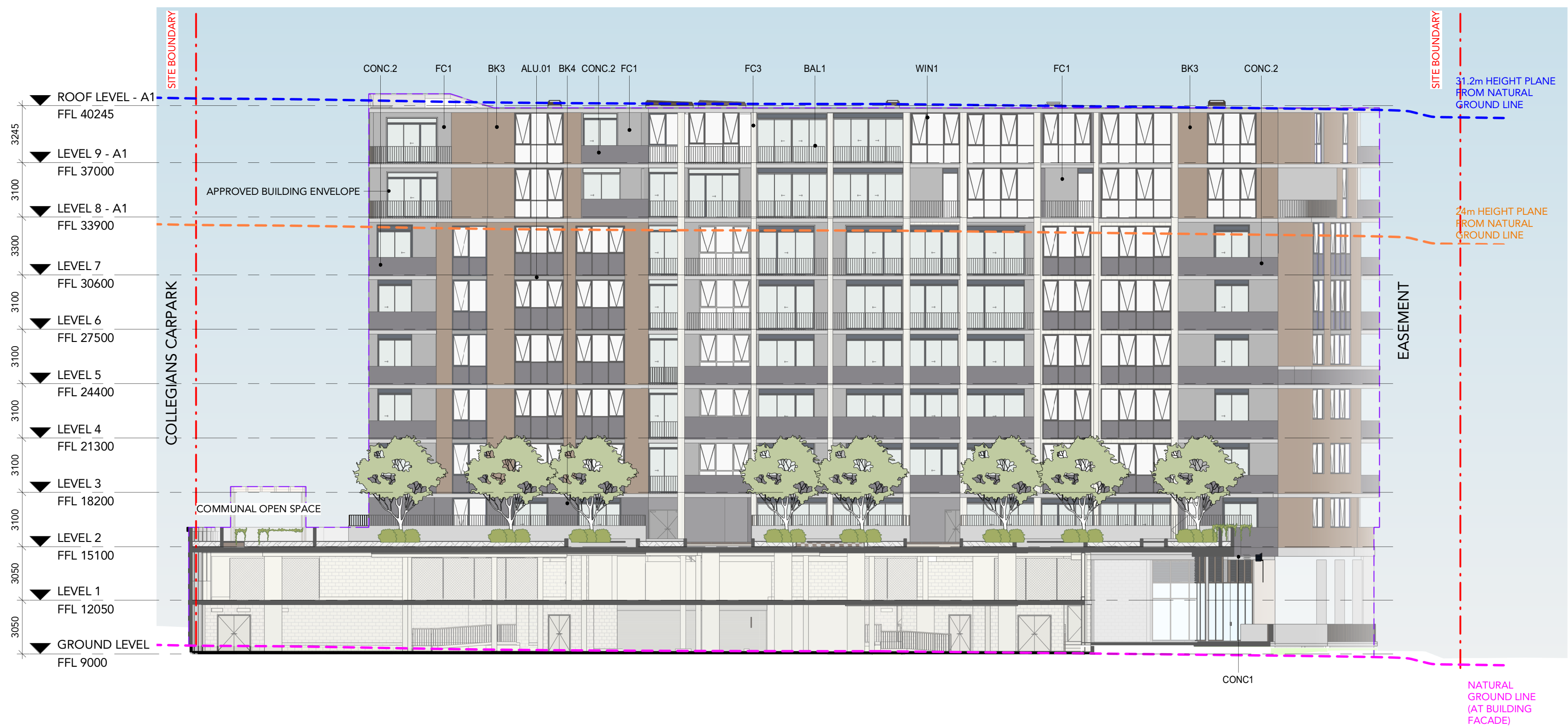
1 NORTH ELEVATION (FROM COMMUNAL SPACE) Scale: 1 : 200
