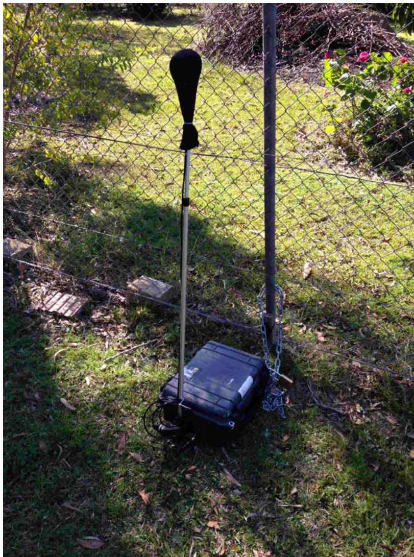
Figure 2 - Example unattended noise logger setup
