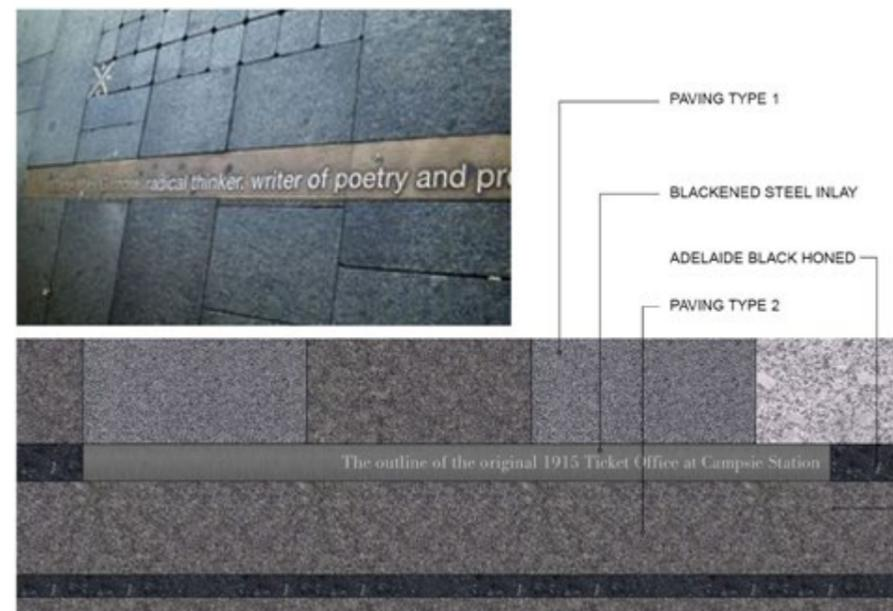
Figure 4.15 Paving inlay detail
