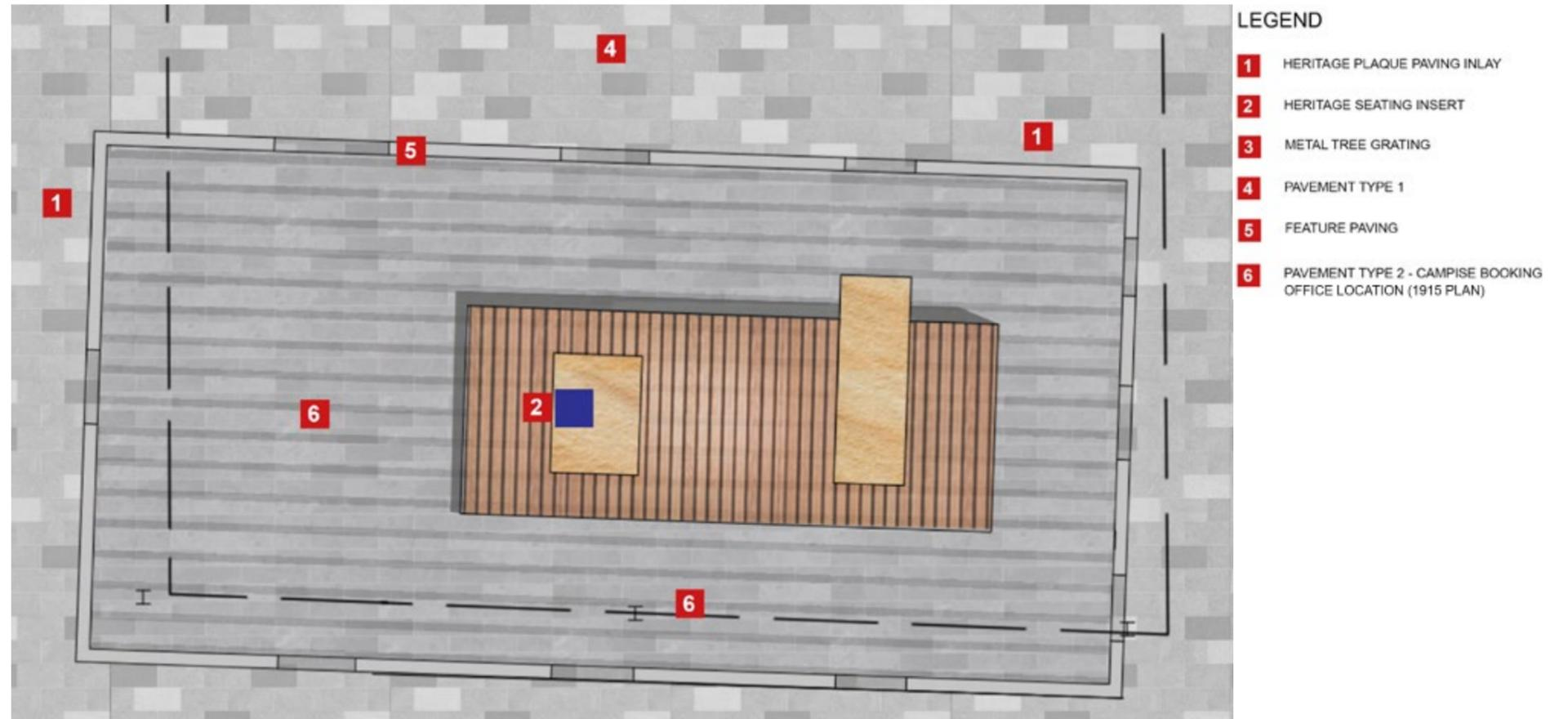
Figure 4.13 Paving inlay and seat element detailed plan
