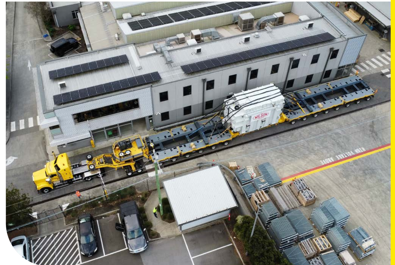
Above: Approximate substation site for transformer delivery shown in red hatching. Below: ARES trailer loaded with Wilson transformer in Glen Waverley.
