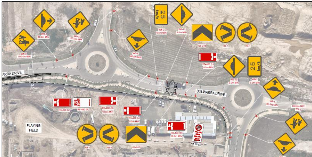
Figure 2-9 Bolwarra Drive Signage
