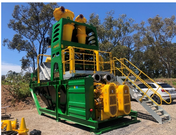
Photograph 1: Example of wash plant (skid mounts to be added, feed tank not shown).
