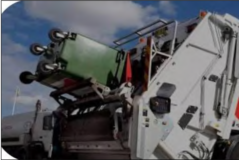
FIGURE 1: EXAMPLE OF THE BIN LIFTING MECHANISIM
