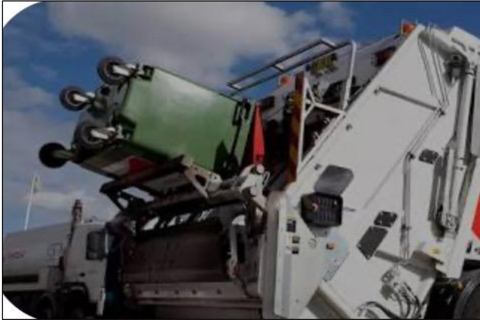
FIGURE 1: EXAMPLE OF THE BIN LIFTING MECHANISM
