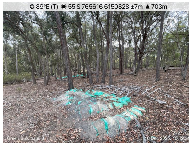
Photo 8: Green bulk bags with soil/rock samples. The plastic has degraded, and the bags are open (16/12/2025)
