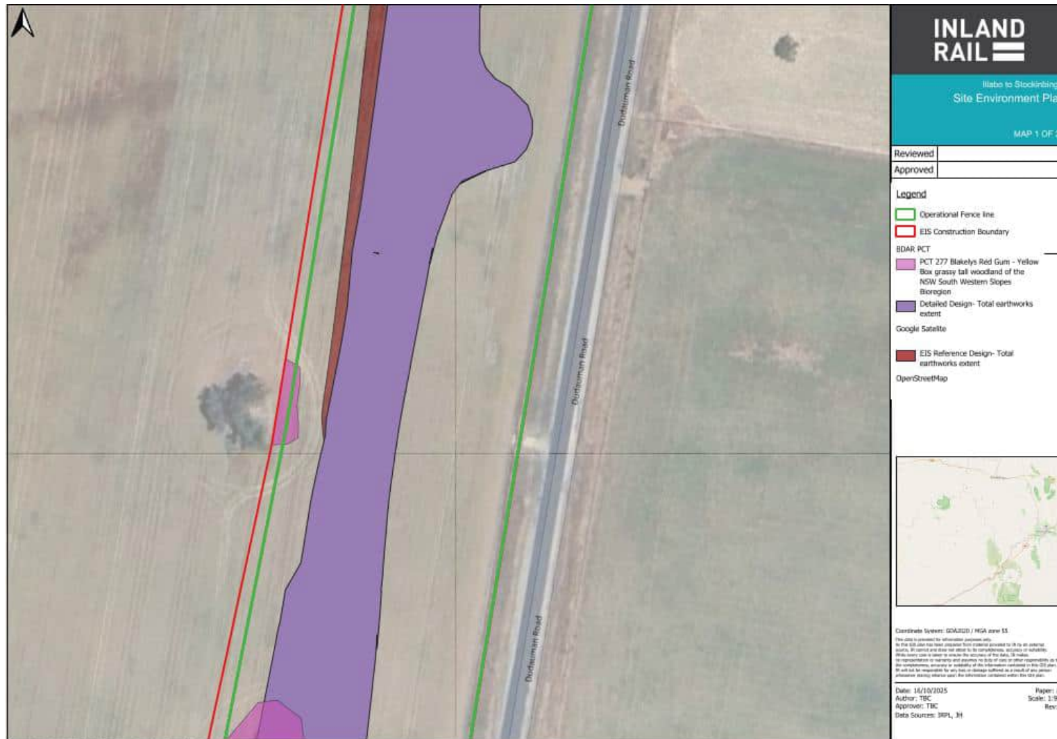
Figure 4-3 Example of reductions in the detailed design earthworks extent from the reference design (reference design in the brown polygon and detailed design in the purple) which has reduced vegetation impacts associated with PCT 277.
