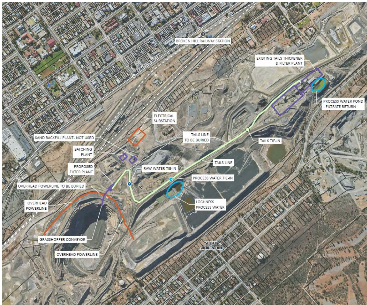
Figure 4 Tailings dewatering system layout
