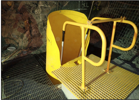
Figure 3: Example of the exit (at the top) of a Safescape Ladder way
