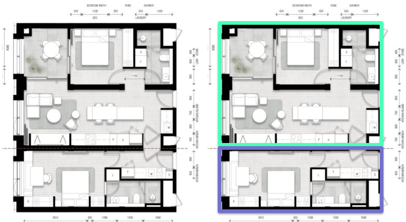
Figure 6 Dual key apartment example arrangement, where functioning as a single apartment (left) and two sole occupancies (one bed and studio) (right)
