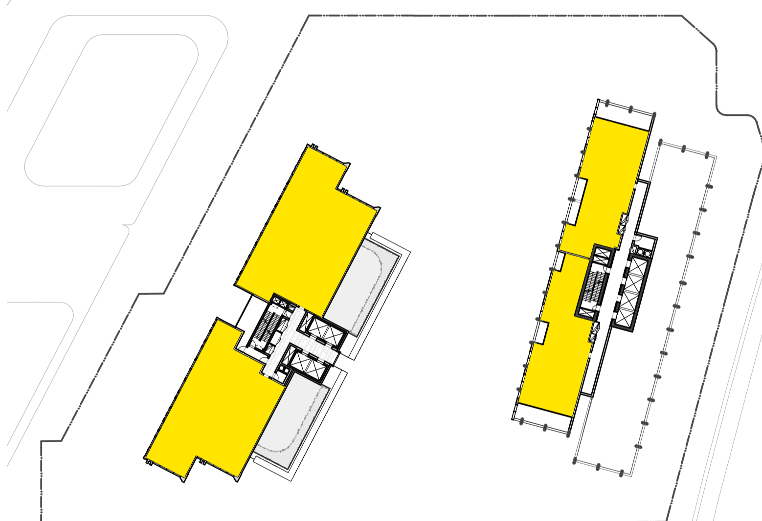
4 SOLAR ACCESS COMPLIANCE L33 Penthouse
