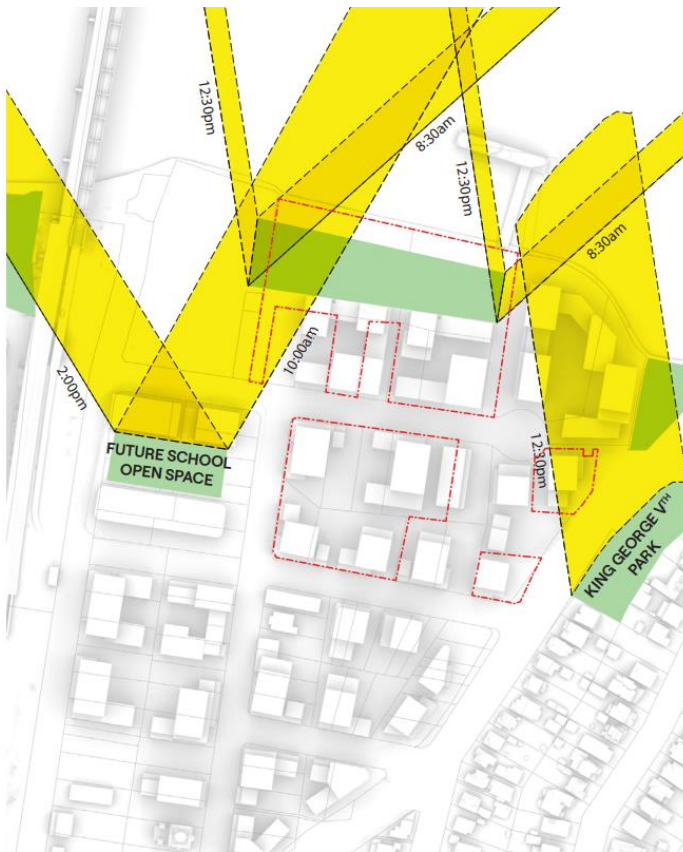
Figure 24 – Solar Access Plane
