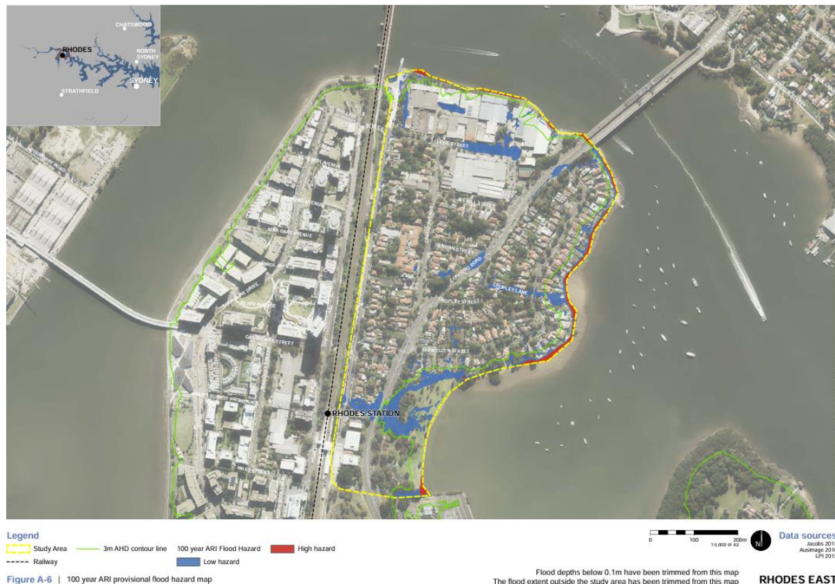
Figure 35 – 100 year ARI provisional flood hazard map
