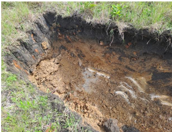
Figure 16: TP4 resulting to bucket and ripper tyne refusal on large colluvial boulders
