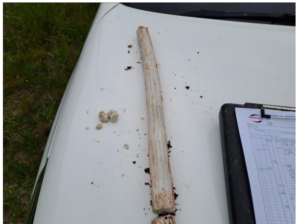
Figure 17: High plasticity, firm kaolinite clay from 7.5m below ground level in BH5
