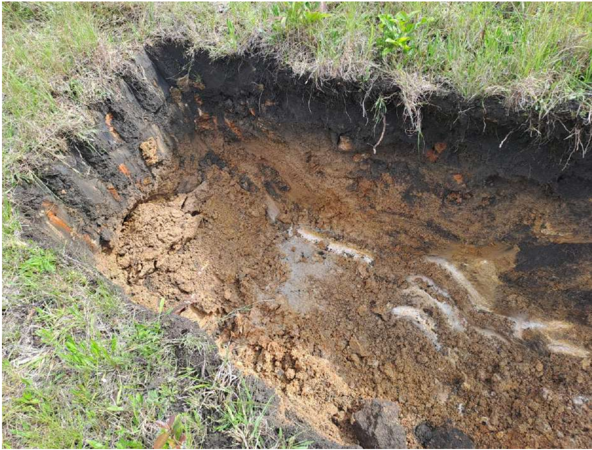
Photograph 5 – Testpit revealing residual/colluvial soils underlying topsoil
