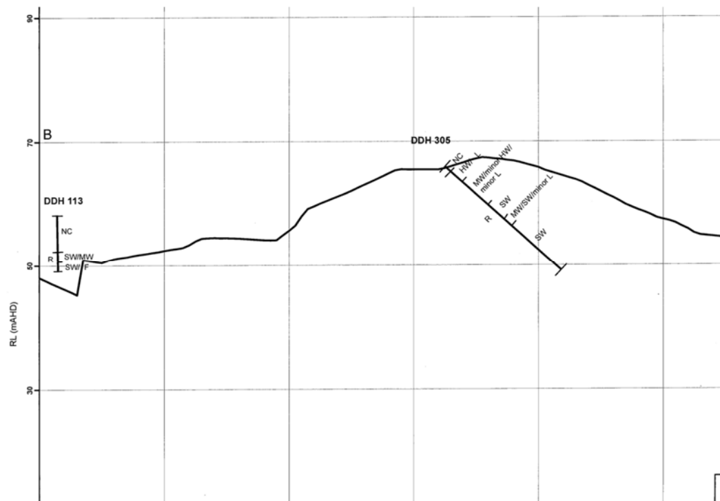
Figure 5-4: Section B Spillway Alignment Interpreted Geology
