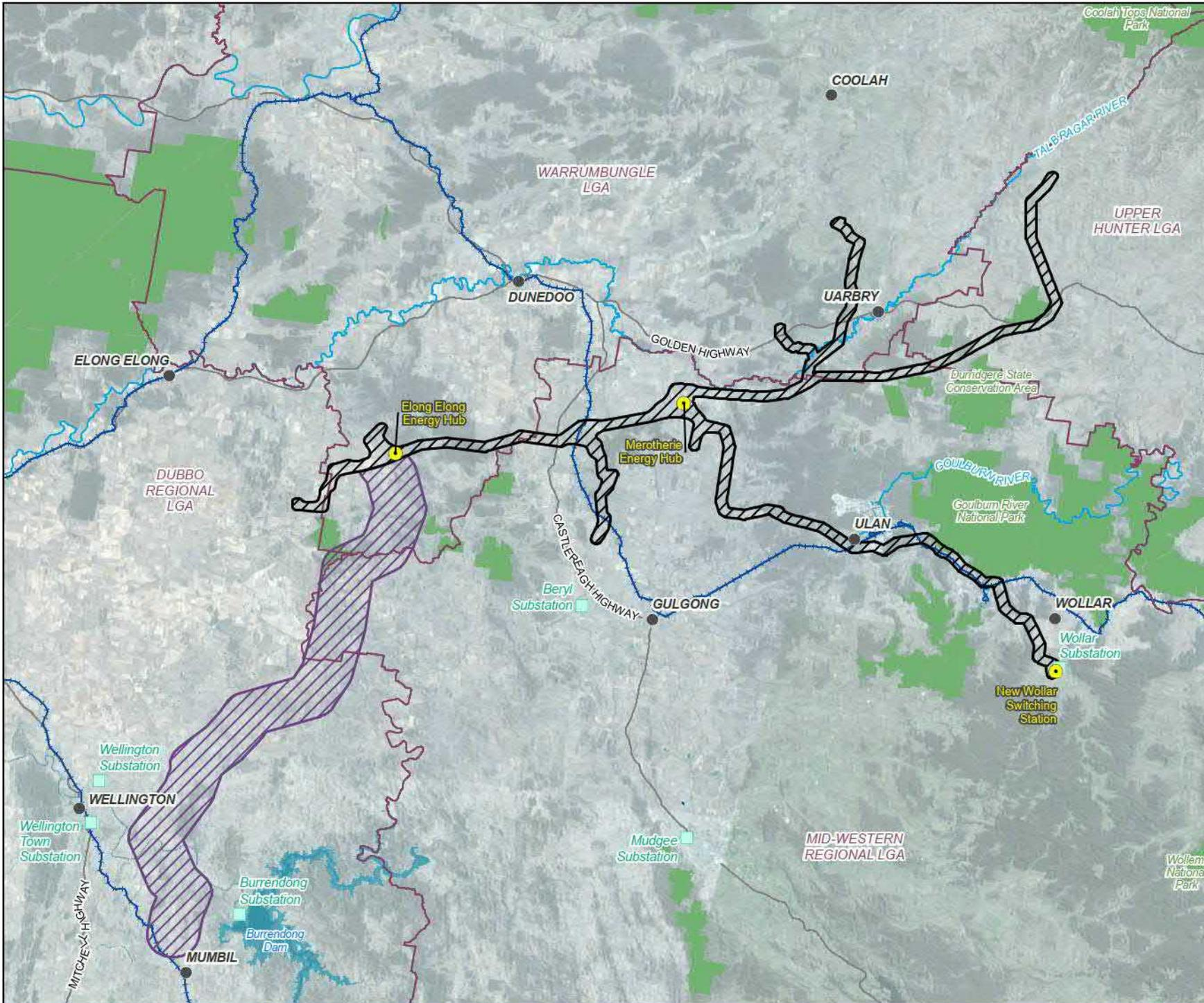
\*The project includes a southern extension of the transmission network between Elong Elong and Mumbil with a connection to the NSW transmission network. This section is under investigation and will be subject to a separate planning approval.
