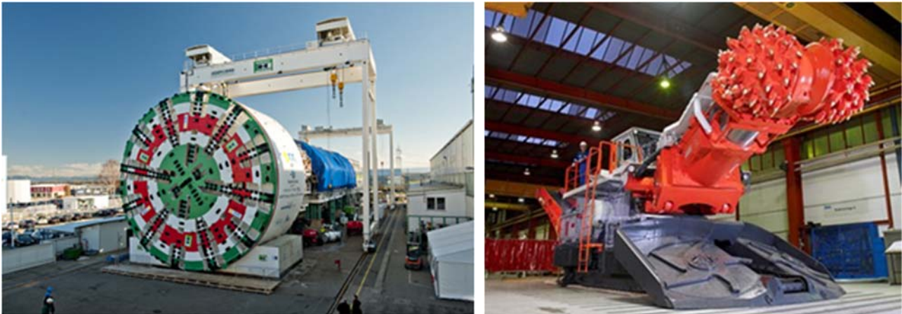
Figure 2-4 Examples of a tunnel boring machine (left) and a roadheader (right)
