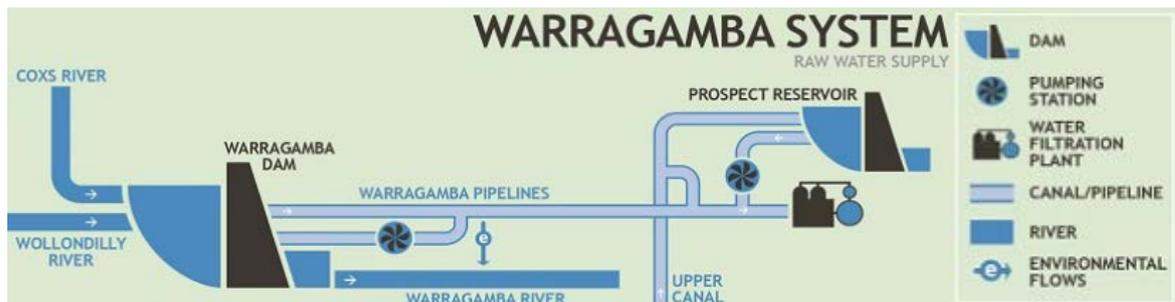
Figure 3-1 Warragamba Water Supply System (Source: WaterNSW)
