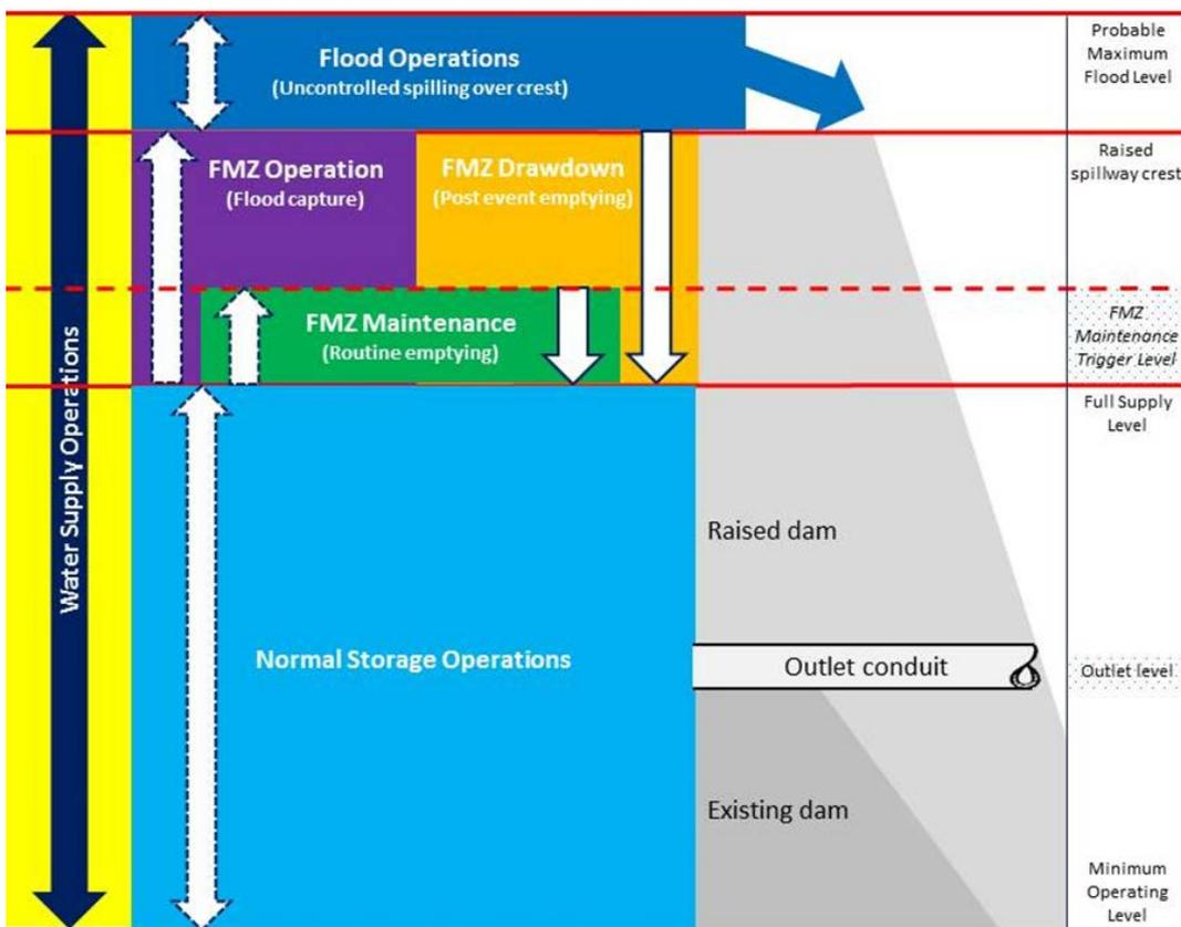
Figure 3-5 Summary of Water Supply Operations for a raised dam – Normal Storage Operations, FSL and FMZ Operation, Drawdown and Maintenance
