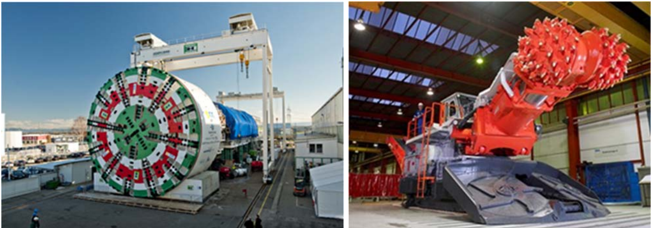
Figure 2-5 Examples of a tunnel boring machine (left) and a roadheader (right)
