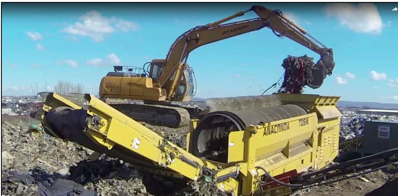
PHOTOGRAPH 3.3 (above): Loading of waste into an Anaconda 516R tracked trommel. The trommel itself is on crawler tracks and can be easily moved if required. To the left and right of the trommel are the conveyors, which deposit processed waste into stockpiles.
