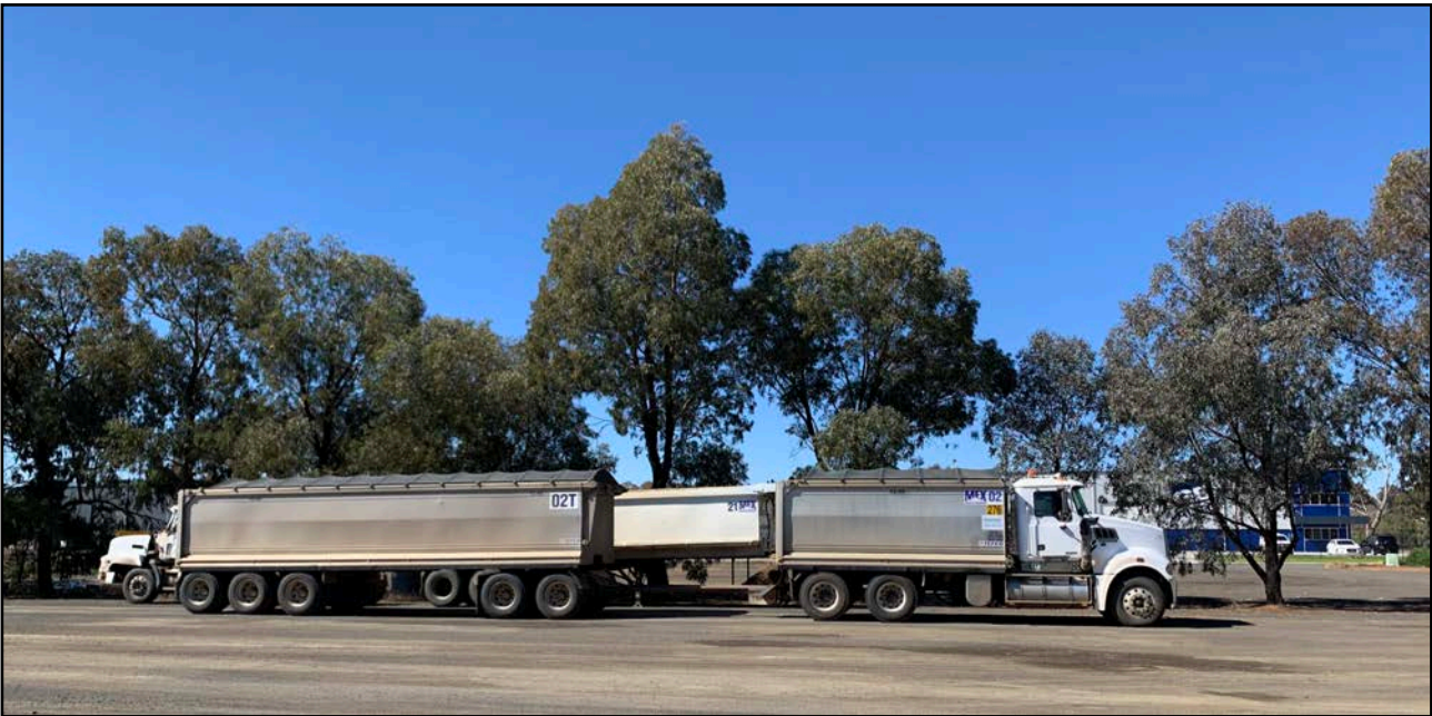
PHOTOGRAPH 3.1 (above): Typical large waste haulage vehicle- 8 axle truck and dog with a current lawful payload of up to 45 tonnes. View of MEX trucks in existing hardstand truck parking area on the project site, with existing landscaping in rear.
