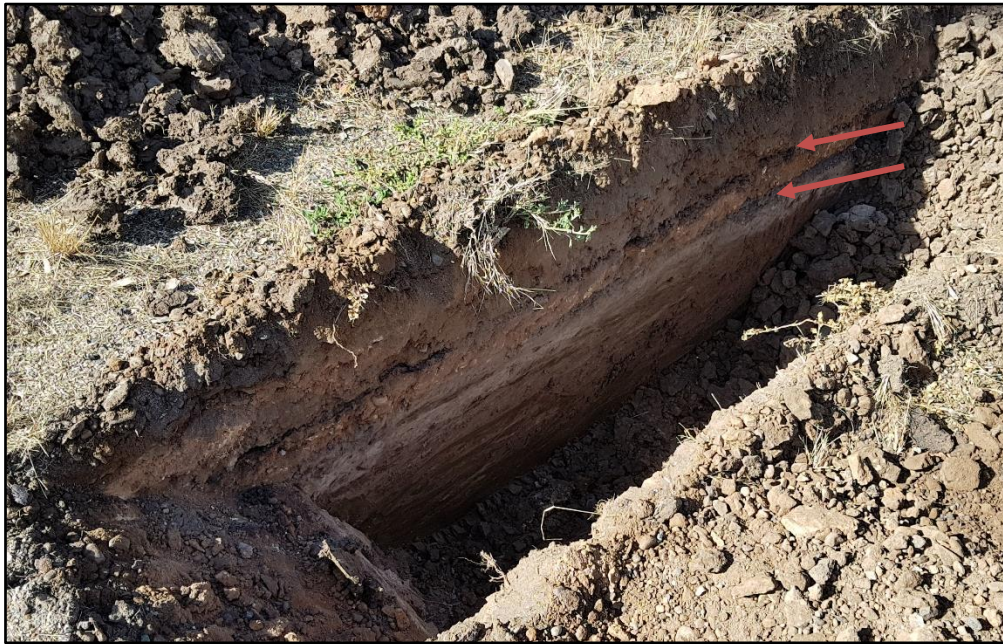
Figure 9: Pit 106 excavation with asphalt layers identified
