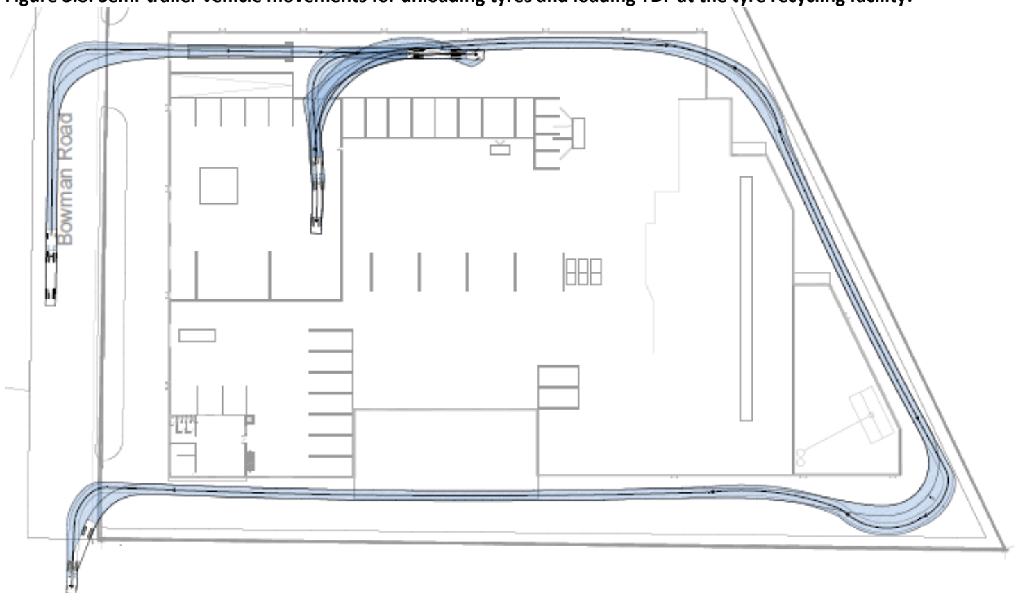
Figure 3.8. Semi-trailer vehicle movements for unloading tyres and loading TDF at the tyre recycling facility.
