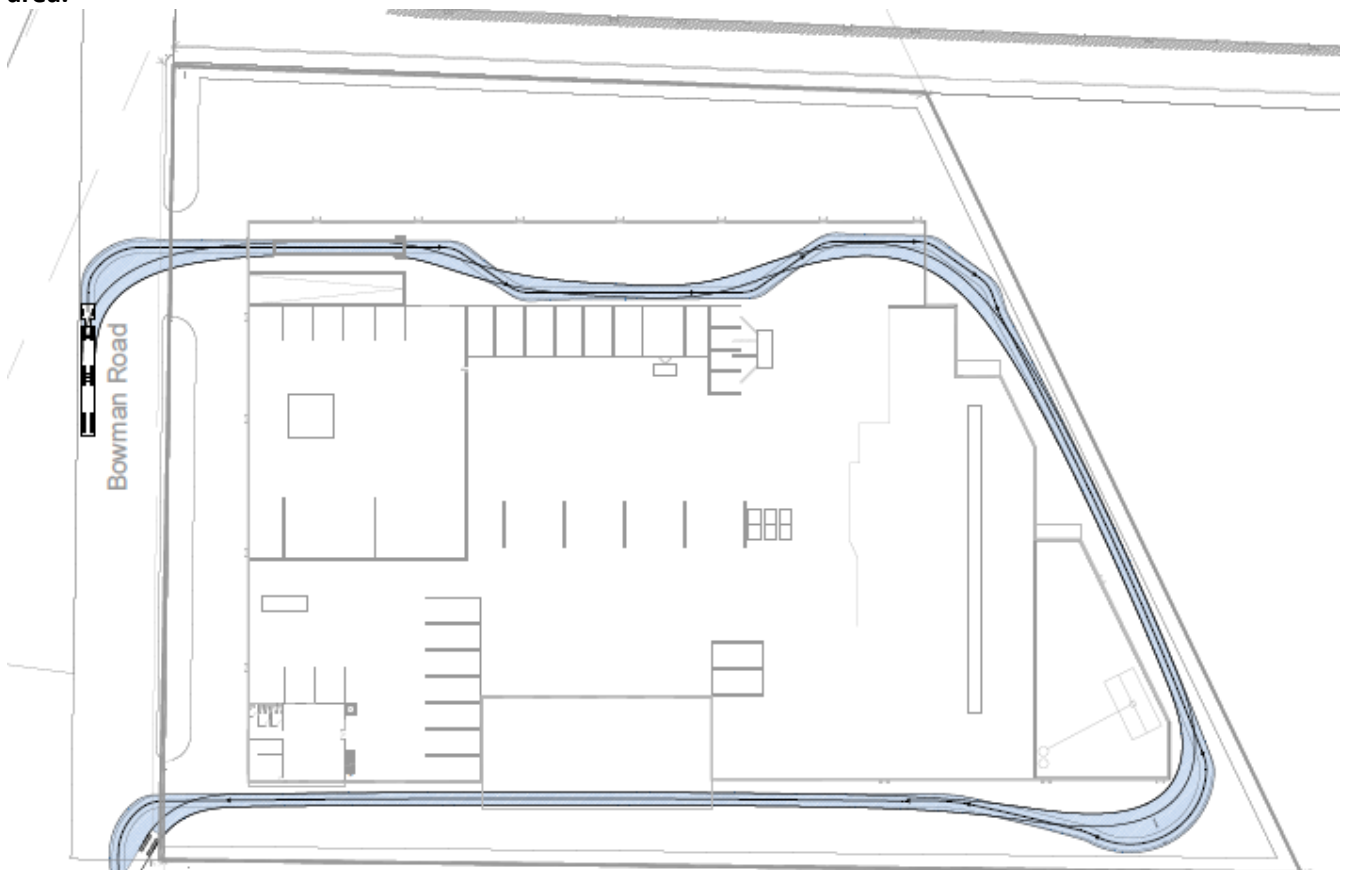
Figure 3.6. B-double vehicle movements for loading recovered products and residual waste at the primary sorting area.
