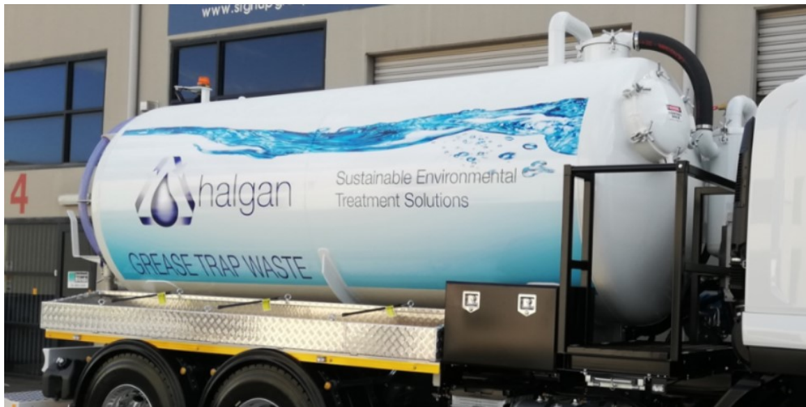
Figure 5.4 Collection Vacuum Tanker (Grease Trap Waste)
