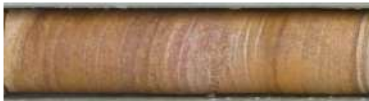
Photograph 2: Typical medium grained coloured sandstone from DMDDH07, sample shown is from 15.1 to 15.4m.
