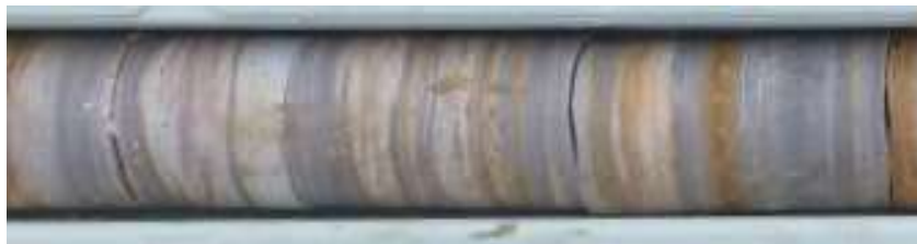
Photograph 1: Ashfield Shale from DMDDH07, sample shown is from 2.45 to 2.80m.
