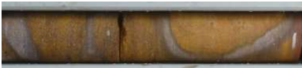
Photograph 6: Liesegang banded ironstone developed in sandstone. DMDDH09, 28.4 to 28.8m. Less often occurring form of ironstone, but often quite thick where it does occur.
