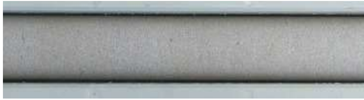
Photograph 7: Yellow Block sandstone, medium grained, very well sorted, massive, photographed on 8 February 2017 just after being drilled. DMDDH07, sample shown is from 57.3 to 57.6m.
