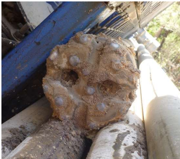
Photograph 11: Reverse circulation down-hole-hammer bit used for percussion holes. The two airways on the bit face are partially blocked as the bit had just been retrieved from a wet ‘muddy’ hole where drill cuttings had pushed into the bit after the air flow had been stopped.
