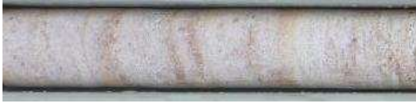
Photograph 3: Typical pale medium-coarse grained sandstone from DMDDH07, sample shown is from 24.15 to 24.5m.
