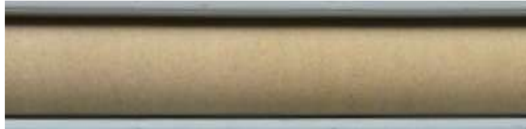
Photograph 8: The same core as in Photograph 7. Yellow Block sandstone photographed on 23 March 2017, six weeks after being drilled. The colour has changed from pale grey to brownish-yellow. DMDDH07, sample shown is from 57.3 to 57.6m.
