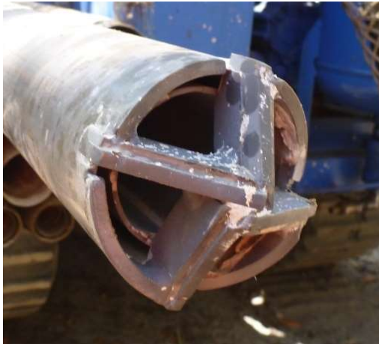
Photograph 10: Aircore bit used for drilling at Maroota.
