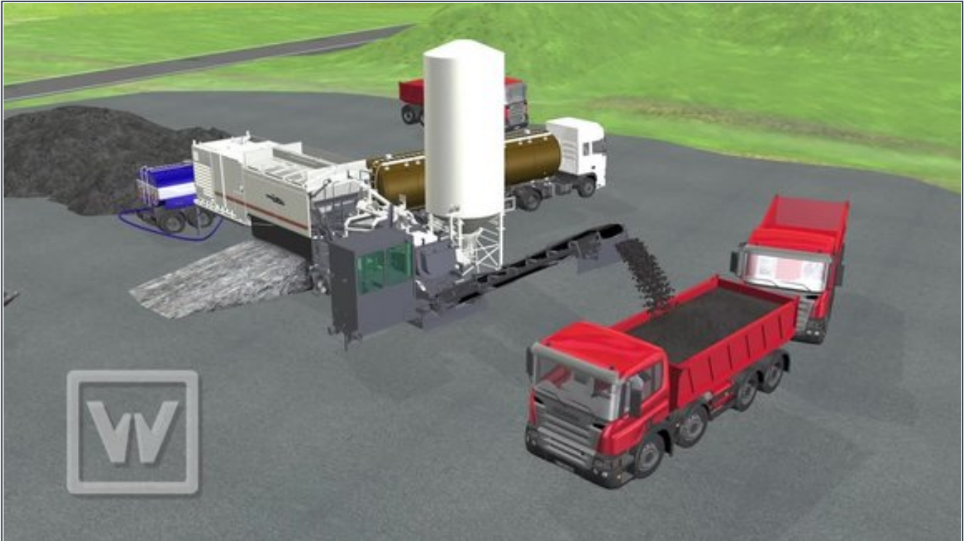
F2.5a: Indicative granular blending plant
