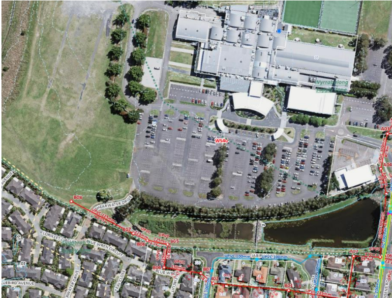
Figure 8: 225mm main on the southern boundary with 25.8ET loading
