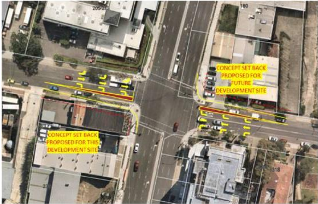
Figure 1: Suggested Setback and Intersection Treatments to better Align Intersection and Increase Capacity
