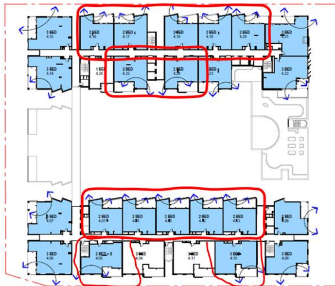
Figure 4. Annotated natural cross ventilation diagram
