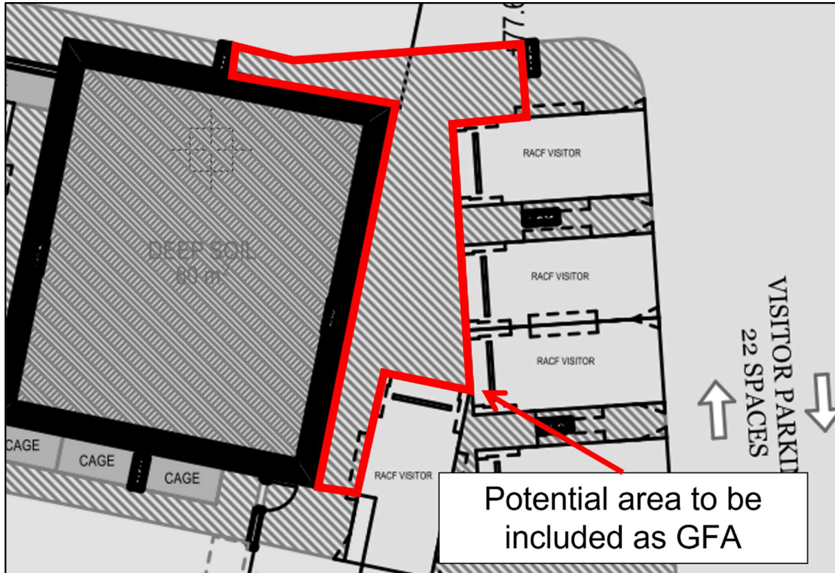
Figure 1 Example of potential area within basement which has no dedicated purpose and may count toward GFA
