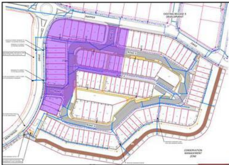
Figure 2. Plan in the June 15 Additional Information showing area in the North West corner of the current site where stormwater will be directed under Montwood Drive (purple highlight).
