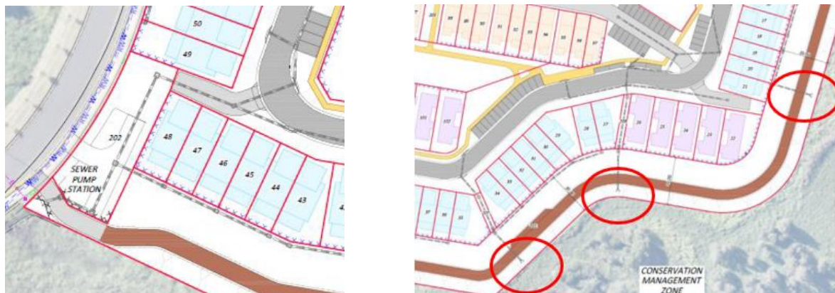
Figure 4. Extracts from Site Plan DWG 140351-S5-DA-AA-01 prepared by NDC dated 15/11/2021. On left hand side there is no HumeCeptor shown, on the right hand side three locations are identified where stormwater will be discharged in the CMZ (circled in red) and no HumeCeptor is shown.
