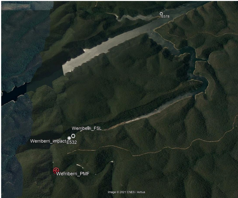
Figure 8. Werriberri Creek: Existing FSL, Impact extent and PMF inundation.
