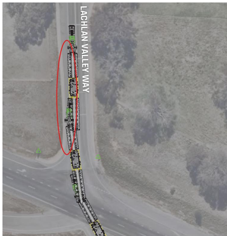
Figure 1: Vehicle chassis on shoulder (indicated with red oval) at Lachlan Valley Way / Hume Highway. Source: Pinch Point 9, OSOM Route Study
