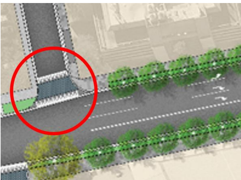
Figure 7: Extract showing required laneway crossing
