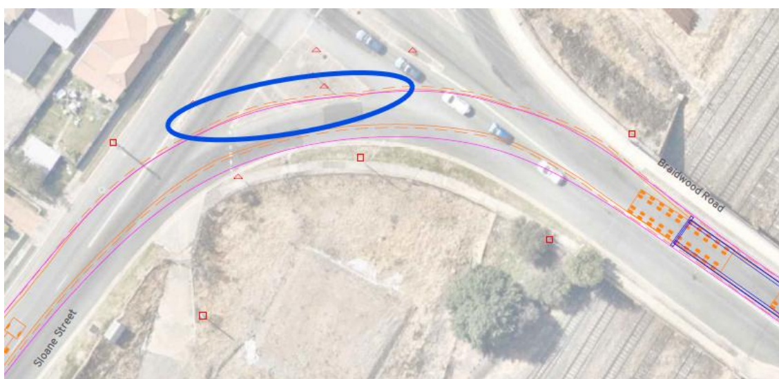
Figure 2: Vehicle chassis outline on raised median (indicated with blue oval) at Sloane Street/Braidwood Road, Goulburn. (Source: Appendix A of TIA)
