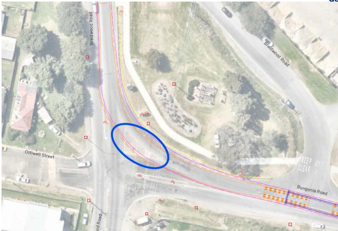
Figure 3: Vehicle chassis outline on raised median (indicated with blue oval) at Ottiwell Street/Braidwood Road/Bungonia Road, Goulburn. (Source: Appendix A of TIA)
